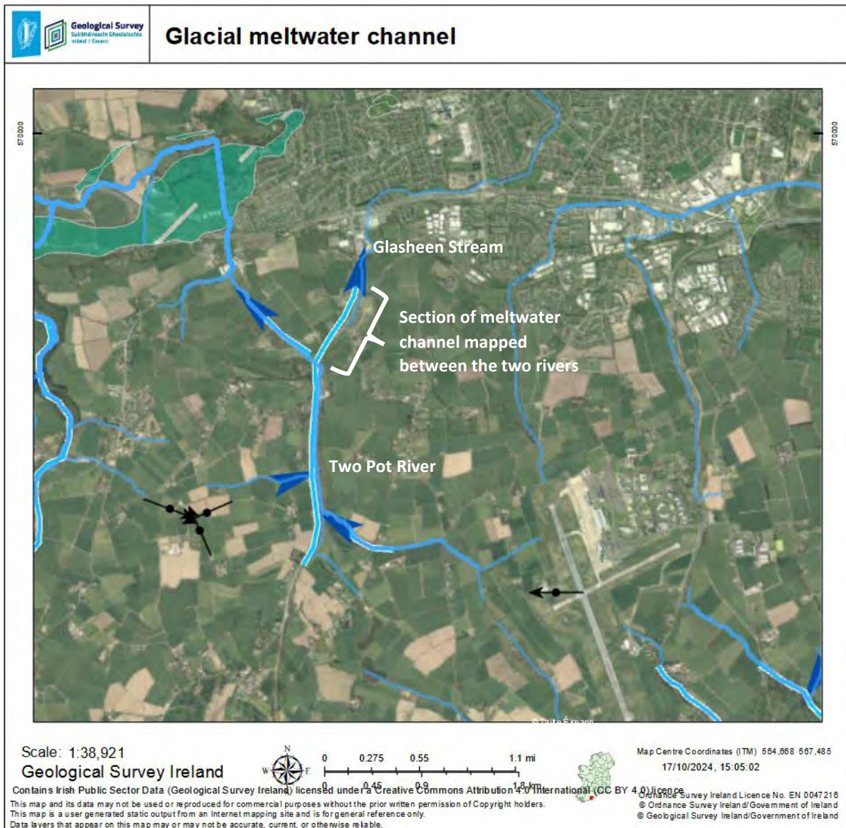
Figure 1-3: Glacial meltwater water channel mapped by GSI between the Two Pot and Glasheen streams. The channel is indicated by the thicker light blue line and blue arrows.
